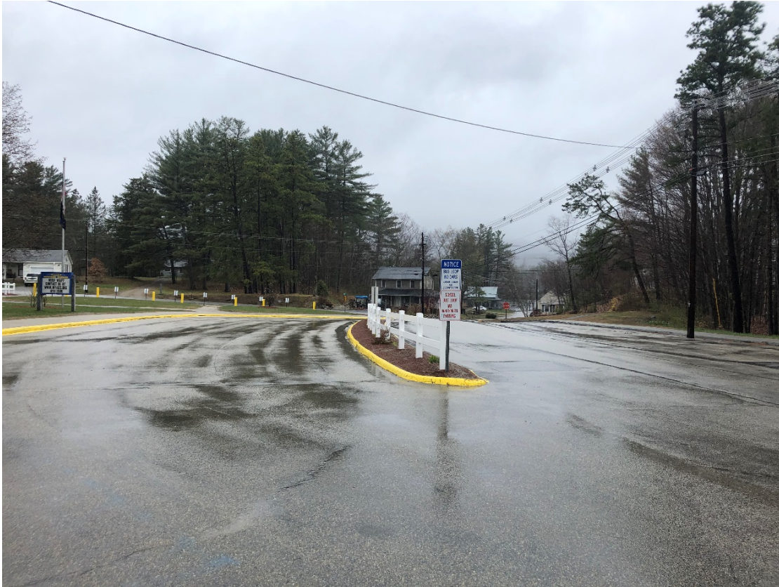
Photo 2. Bus drop off/pick up area at Alton Central School. Road width exceeds 30 horizontal feet and provides an opportunity for pavement reduction and simple flow-in/flow-out bioswale system.
