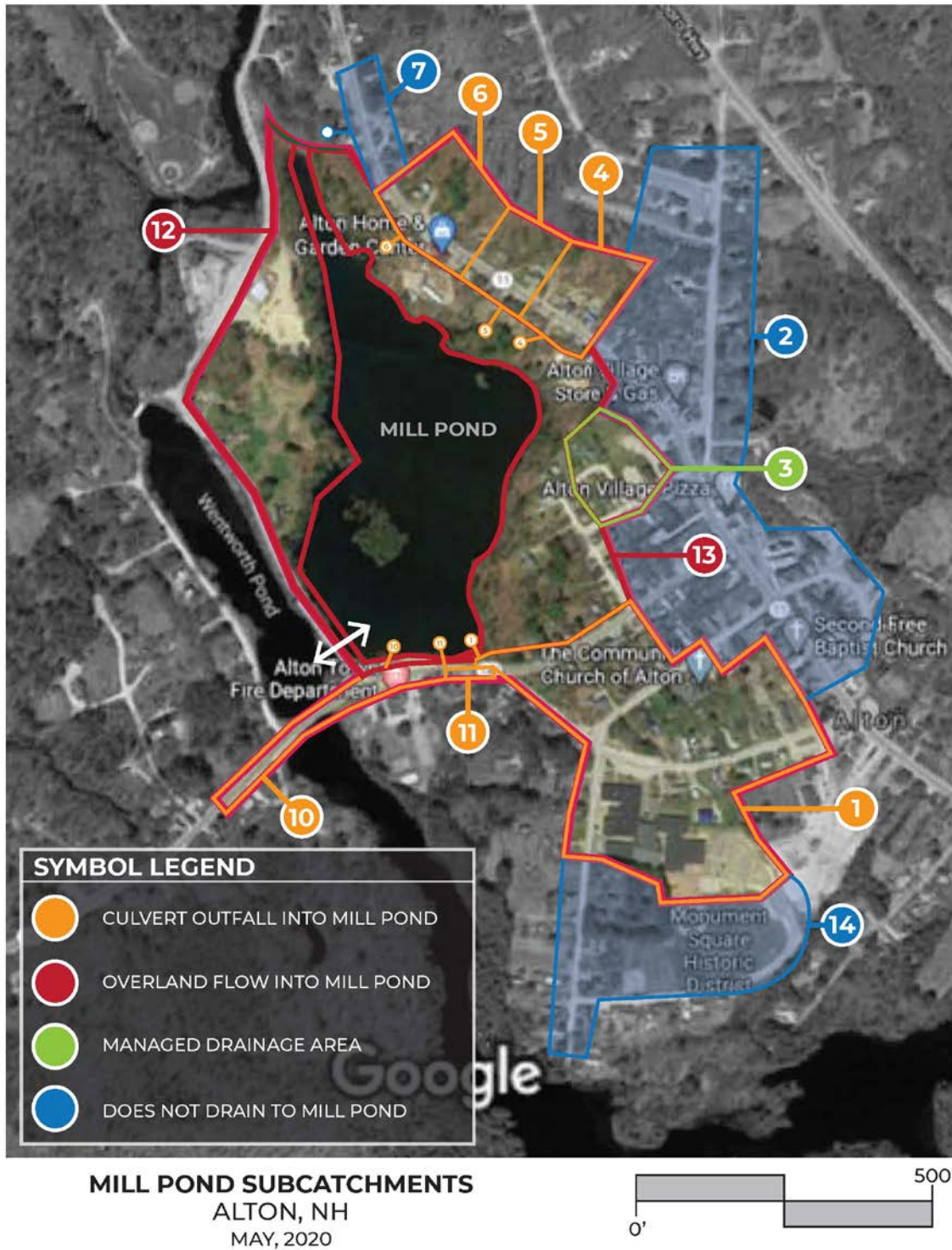
Figure 1. Subcatchment Areas Draining to Mill Pond. Subcatchments 8 & 9 are north of subcatchment 7 and do not contribute runoff to Mill Pond.
